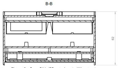
Figure 2 - PoweDIN 4PZ cut view (millimeters)
