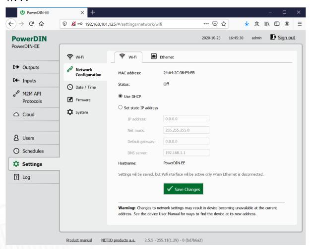
Figure 39 - Network configuration - Wi-Fi
