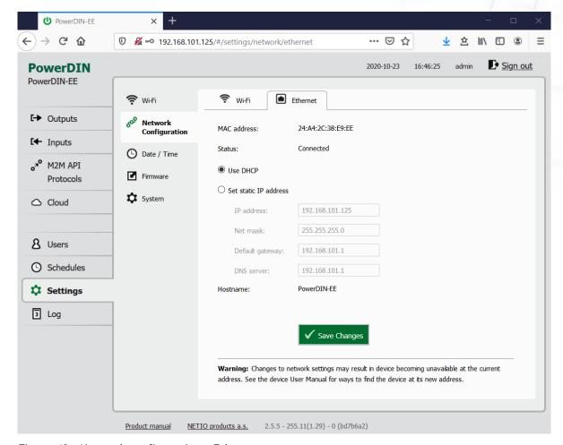
Figure 40 - Network configuration - Ethernet
