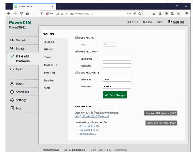
Figure 23 - XML API protocol configuration
