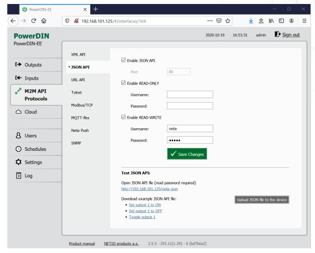
Figure 25 - JSON API protocol configuration
