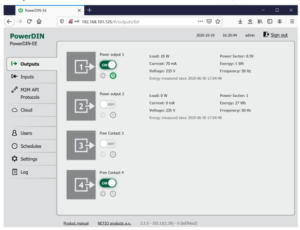
Figure 16 - Controlling the output
