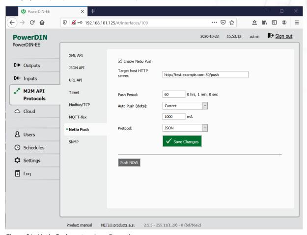
Figure 31 -Netio Push protocol configuration
