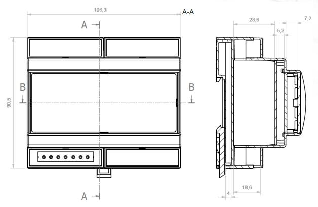
Figure 1 - PoweDIN 4PZ front and side view (millimeters)
