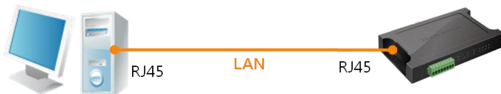
Figure 2-1 the connection between CIE-H14 and a PC
